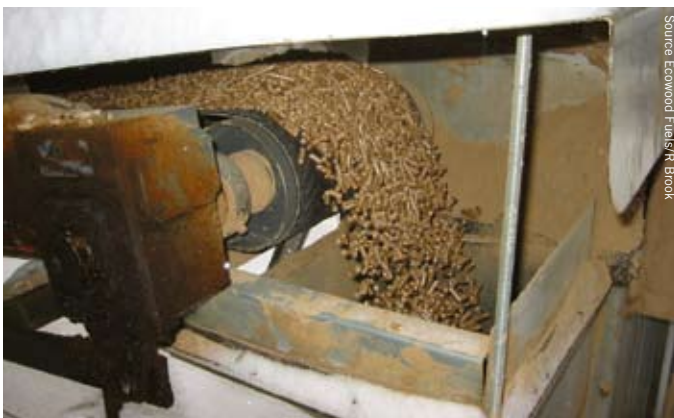
High quality finished pellet coming off the production line in readiness for bagging or bulk storage
