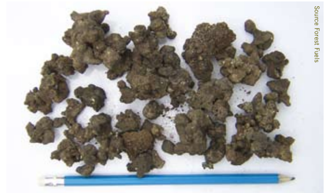
Clinker – glass like substance created as ash melts resulting in damage to the boiler grate
