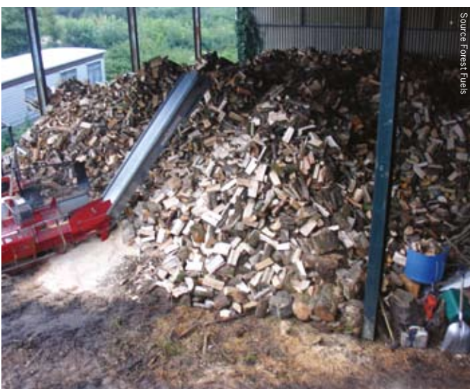
Automated log production using a low cost processor and mini tractor, with direct storage into and open barn for seasoning
