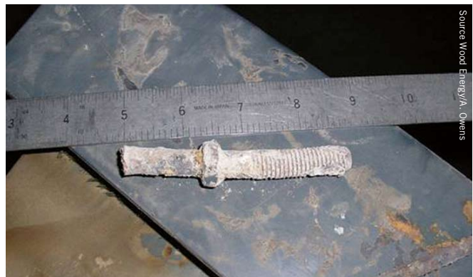
Metal contamination and stones found in boiler system supplied from arboricultural arisings and recycled material
