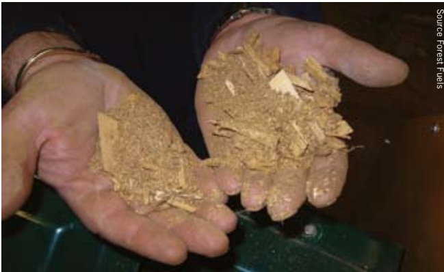
High level of dust in woodchip – very dry woodchip with dust has the potential to cause clinker due to high boiler temperatures unless regulated by exhaust gas recirculation
