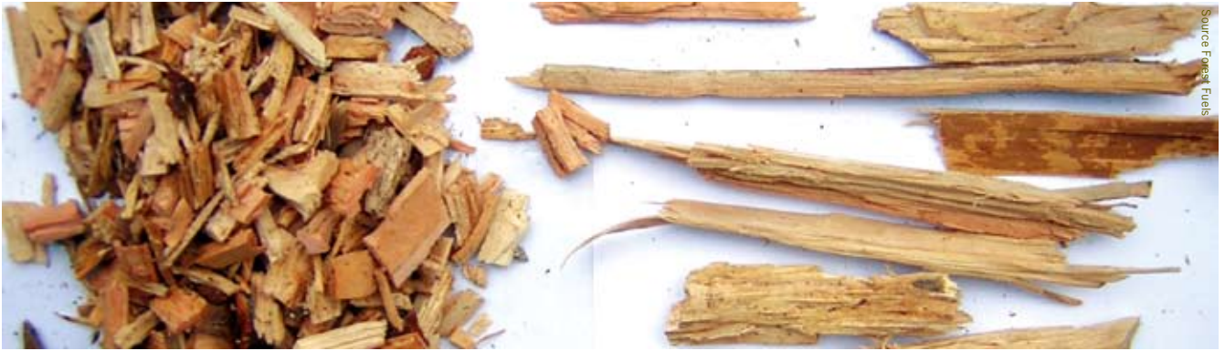
G30/P16 – W30 specification woodchip oversize material/shards
