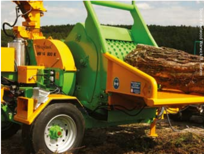
Heizohack Drum Chipper – Heizomat are a German biomass boiler manufacturer who began manufacturing chippers under the brand Heizohack because of the limitations of many chipper in the market to produce Fuelwood.
