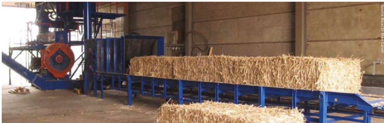
Baled miscanthus being fed into pellet plant for conversion into fuel cubes.
