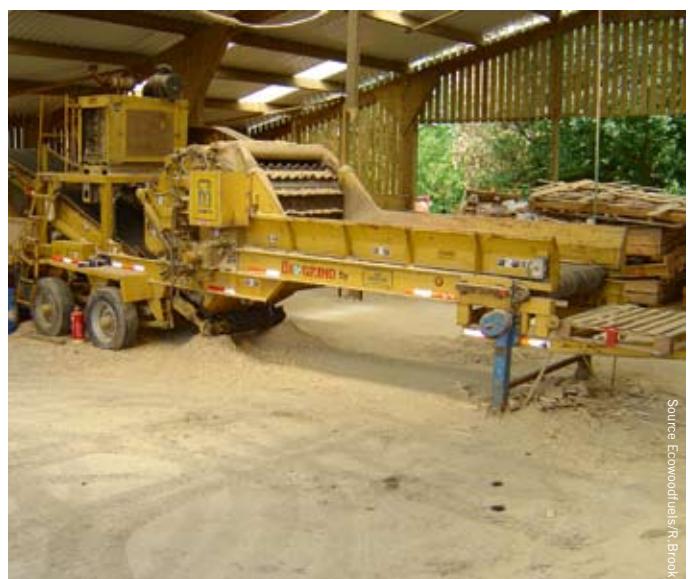
Shredder used for pellet production, material can be re-circulated to improve the quality of the finished product
