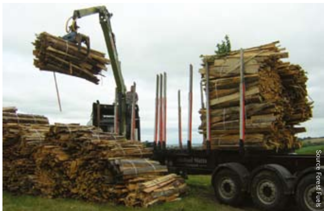
Slabwood stacked for drying in an open exposed location orientated to allow the prevailing wind through the stack at 90 degrees
