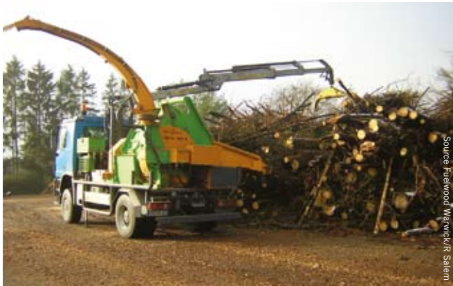
Heizohack Chipper 14-800 purpose built lorry mounted chipper with seven metre reach grab—working with whole trees at roadside
