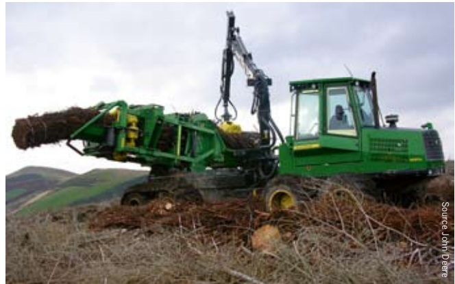
Baler producing log bundles of harvesting brush, ready for transportation and then chipping
