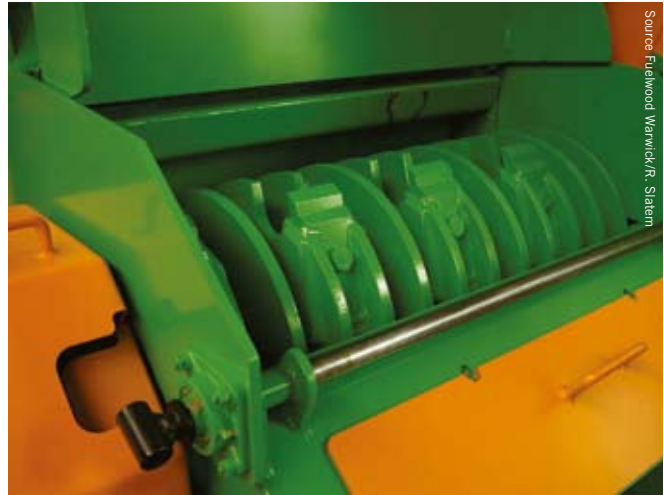
Internal view of drum chipper showing blade settings.
