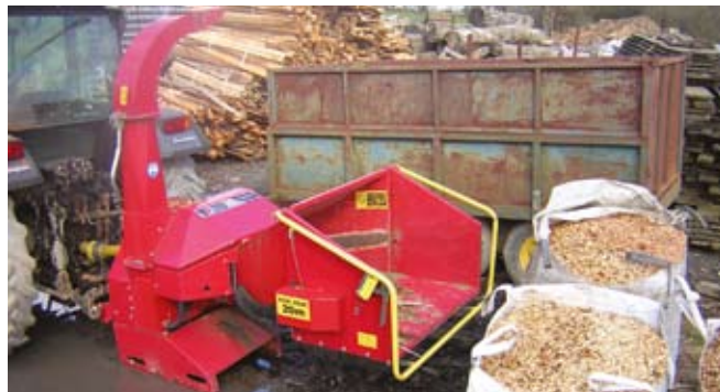
Disk chipper – most common type of chipper on the market today, used widely by tree surgeons
